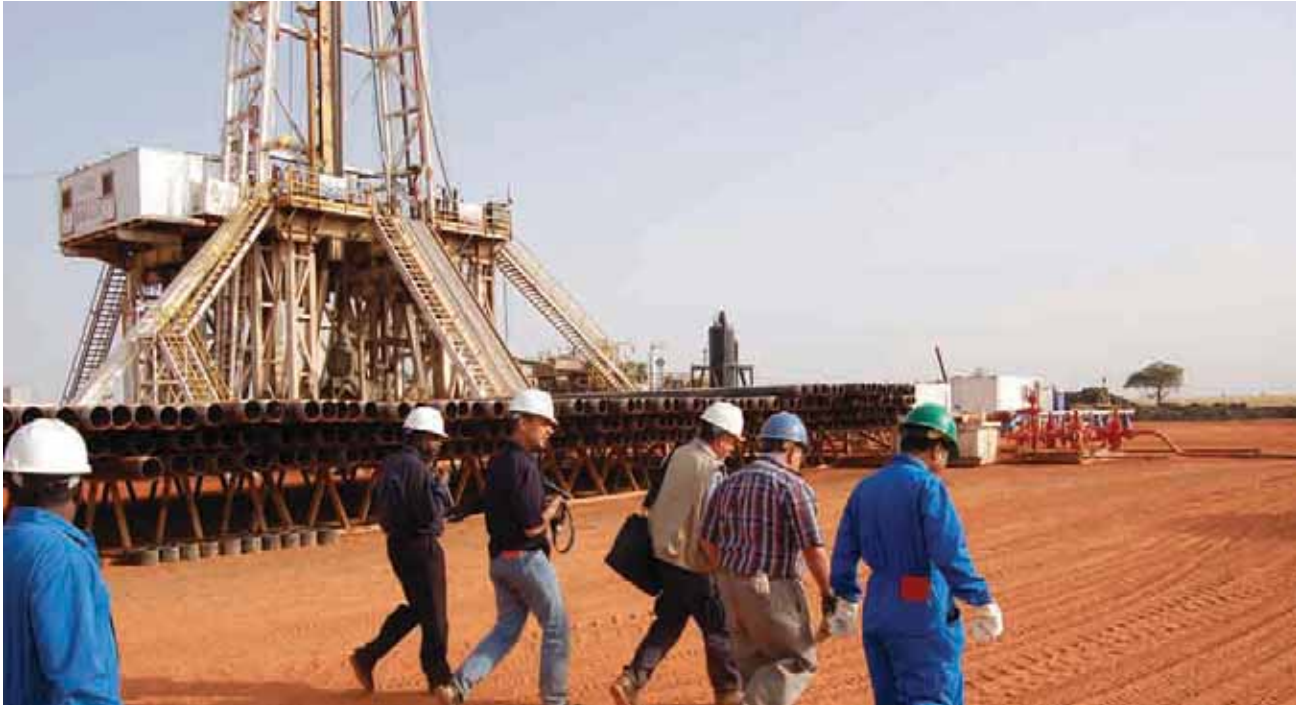
Well casings lined up beneath a Heglig drilling rig in South Kordufan. ©UNEP
