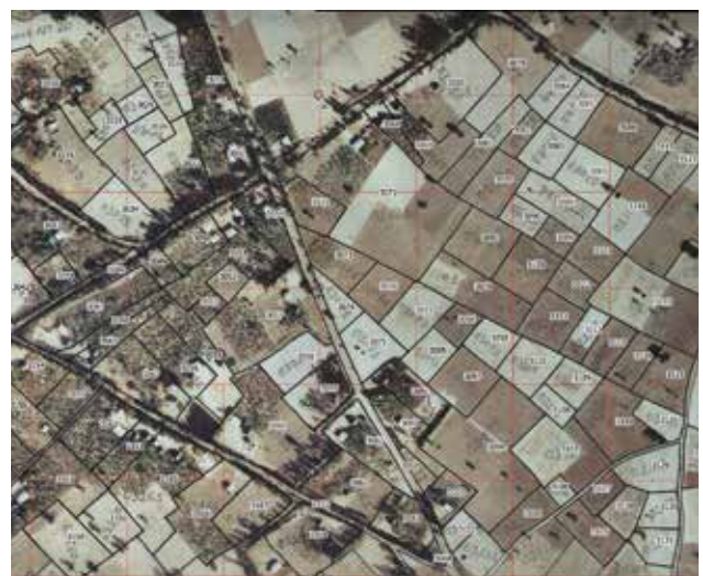
Map 4.2: Building the spatial framework. Left: Aerial imagery used as a field work map sheet with a georeferenced grid. The map shows the delineated parcel boundaries and parcel identification numbers. Right: A vectorised field map showing the resulting cadastral map with parcel boundaries. Source: Zerfu Hailu, Ethiopia.
